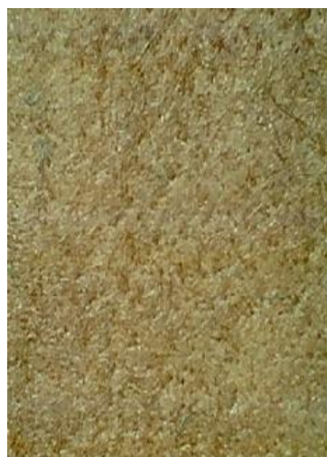
Figure 8: Jute Felt of 12mm thick and GSM 1650 used as a glu core
