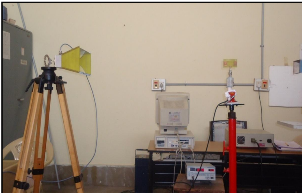
Figure 5: Turn table and PC based radiation pattern measurement setup and photograph
