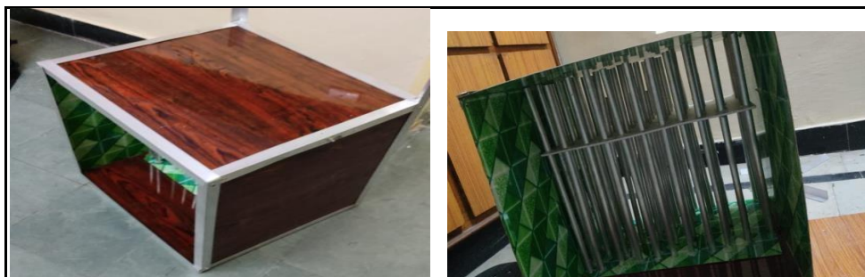
Figure 3: PCM based air cooler in different orientations.
