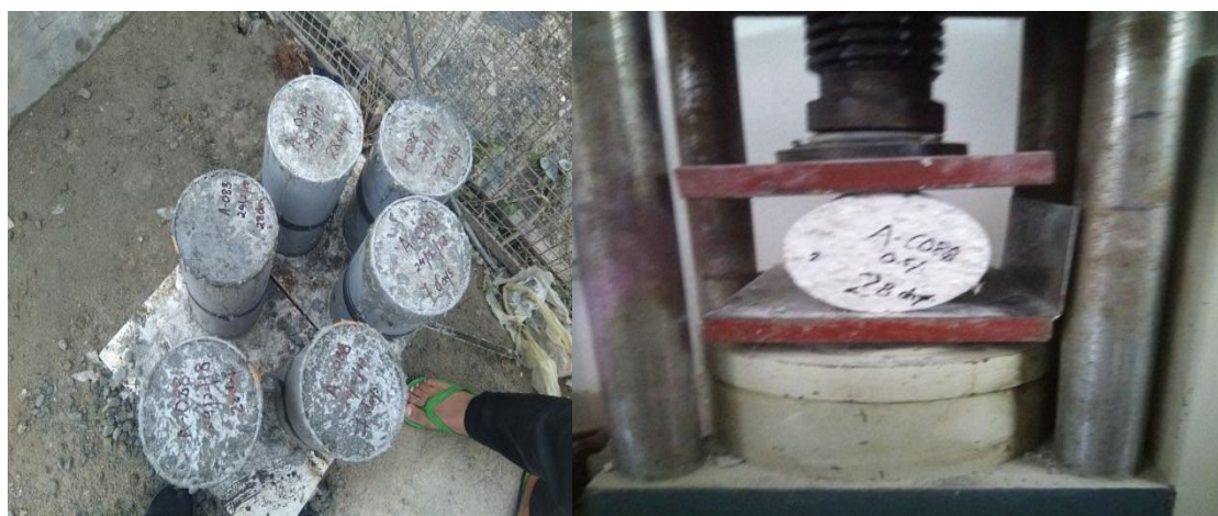
Figure 5 : Testing of cylinder specimens.
