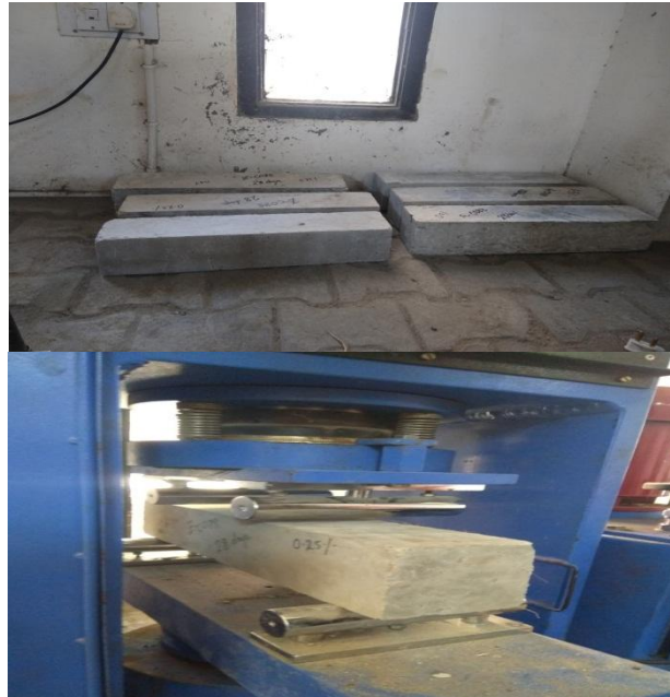
Figure 4: Testing of beam specimens.
