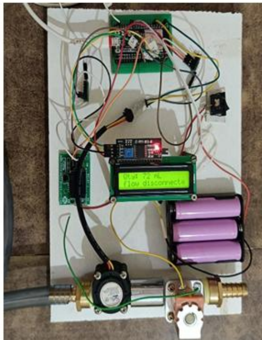
Figure 12: Model Image with Flow Disconnected
