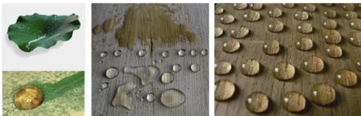
Figure 2: The Lotus Effect and Waterproofing Provided by Silica Nanoparticle-based Nano-Coatings on Wood Surfaces (Marzi, 2015)
