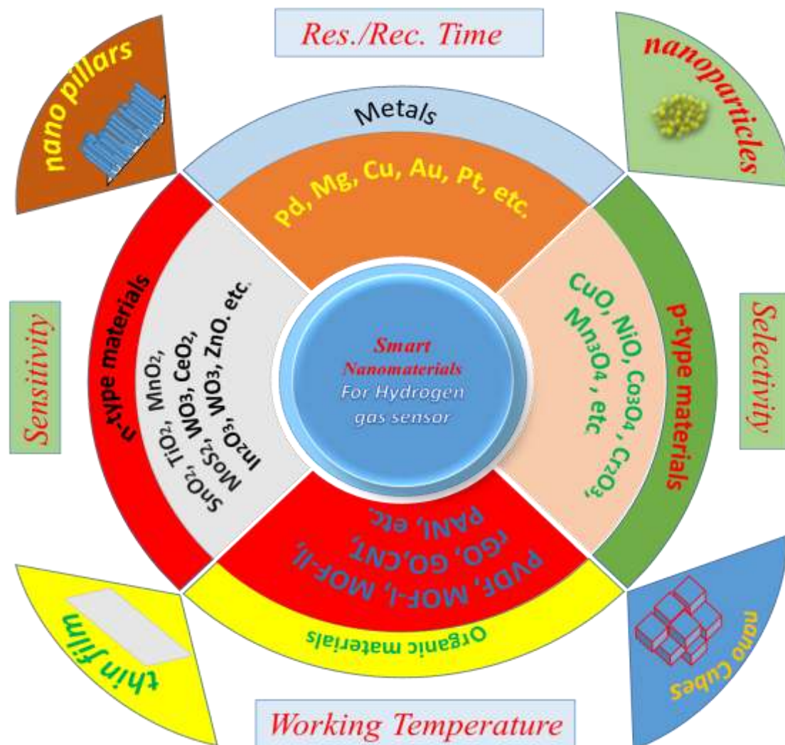
Figure 1: Shows different advanced nanomaterials for fabricating reliable hydrogen gas detection sensors.
