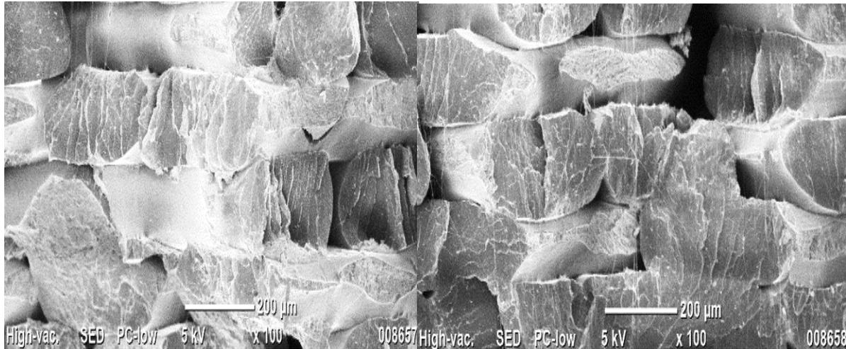
**Figure 4.3:** SEM images of fractured interface of (a) PLA (b) ABS
