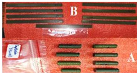
**Figure 3.5:** Printed samples a) Compression
