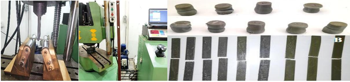
**Figure 3.6:** a) Flexural b) Compression
