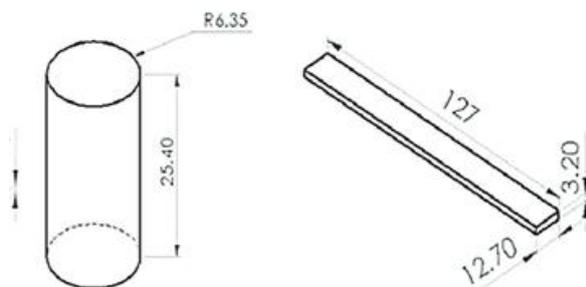
**Figure 3.2:** a) Compression b) Flexural specimen
