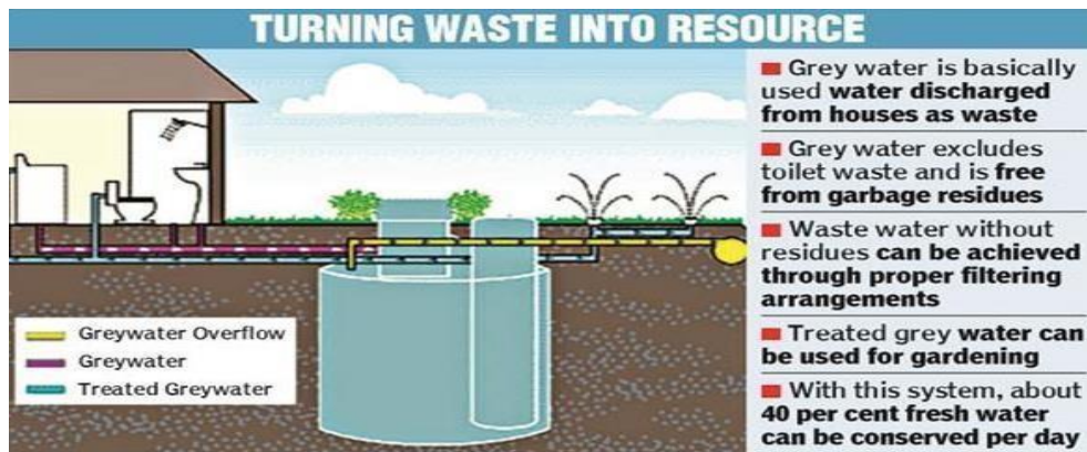
Figure 2: Grey water purification [32]
