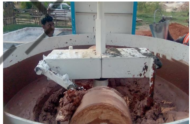
Traditional lime mortar mill with adjacent slaking tank
