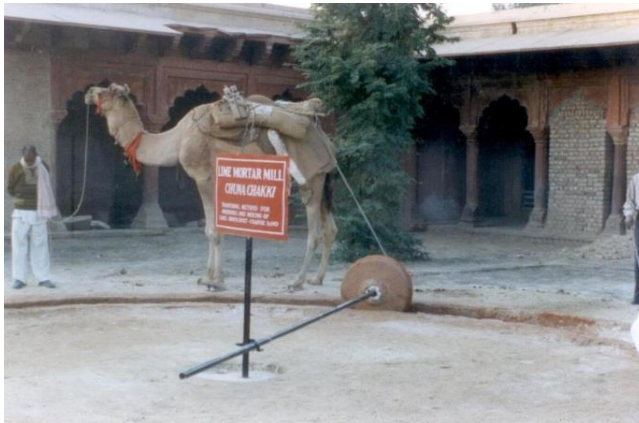
Figure 5: Traditional lime mortar mill (camel)
