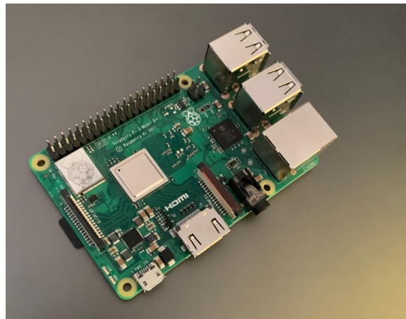
Figure 2: Raspberry - Pi 3 B+
