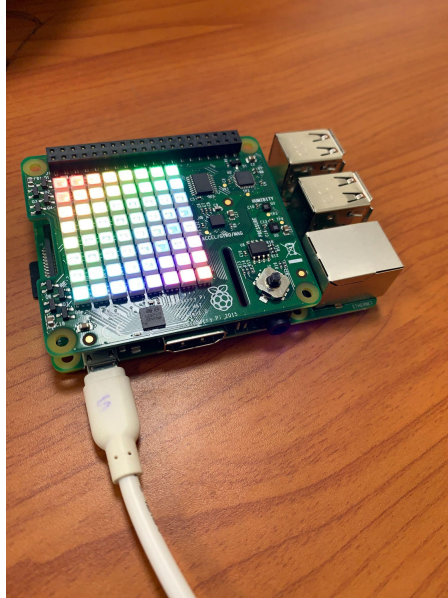
Figure 3: Raspberry-Pi Sense HAT
