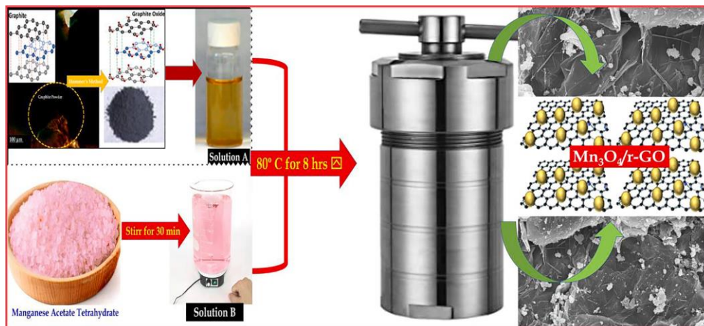
Fig. 9. Schematic illustration of the synthesis of Mn 3 O 4 -rGO NCs (Ref.15)
