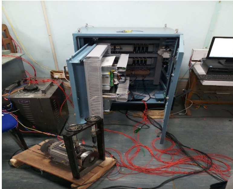
Figure 3. Micro-grid prototype with various loads connected to the PMU
