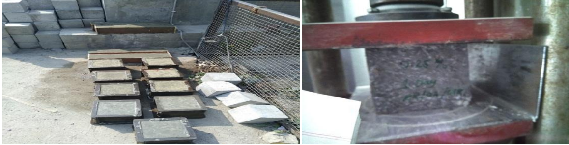
Fig.3 Testing of cube specimens.
