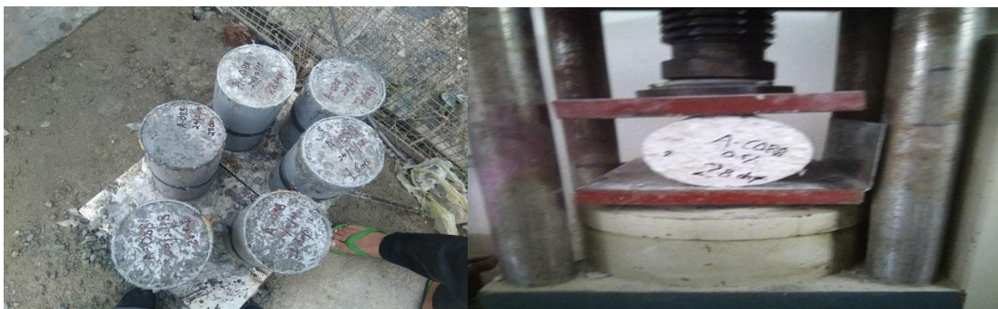
Fig.5 Testing of cylinder specimens.
