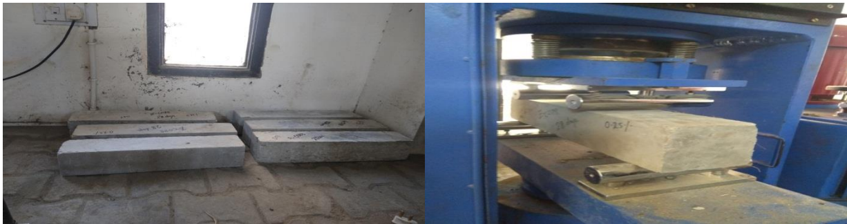
Fig.4 Testing of beam specimens.
