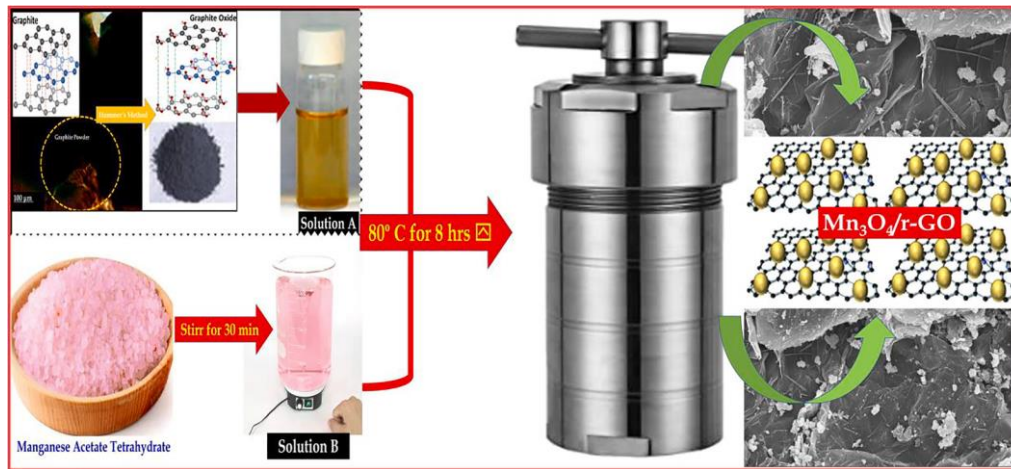
Fig. 9. Schematic representation of the synthesis of Mn_3O_4 -rGO NC (re-printed from Ref.15)
