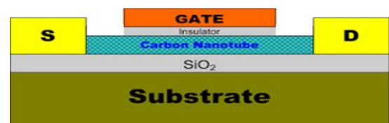
Fig.2. Schematic figure of a CNTFET
