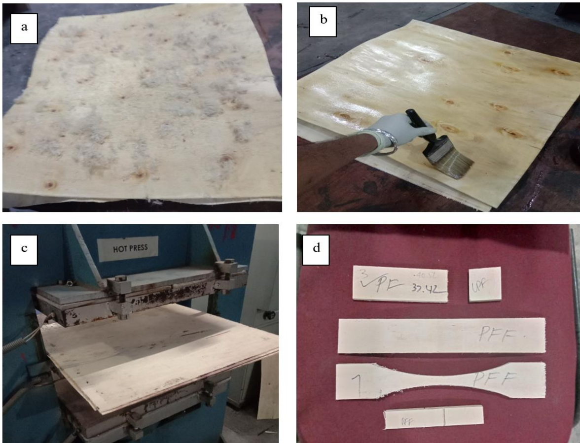
Fig. 1 Short hemp fibers and veneer assembly [a], resin application by using brush [b], plywood assembly for hot pressing [c], test specimens [d]
