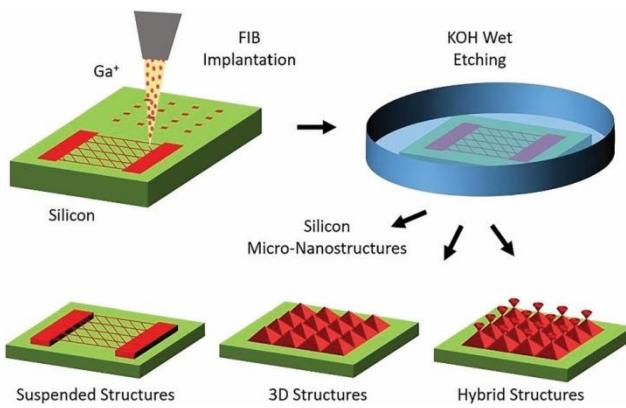
An illustration showing how bulk Si structuring with an ion beam can be used to create 3D micro-nanostructures. This involves anisotropic wet etching in KOH solution, anisotropic implantation in Si using Ga FIB lithography, mask writing at nanometer resolution, and fabrication of Si micro-nanostructures by selectively removing the un-implanted region.
