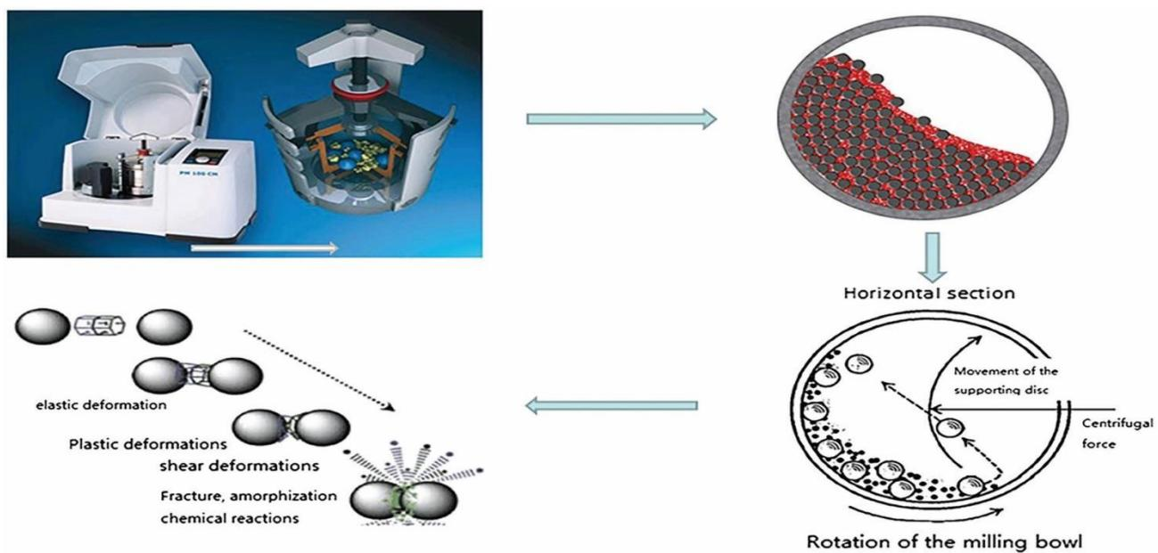
The ball milling method's basic idea. Reprinted from ref. 25 with permission. John Wiley & Sons, Ltd., 2016-2017.
