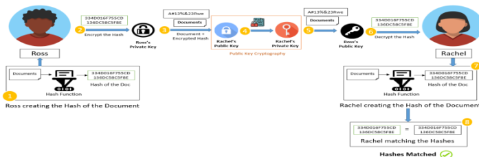
FIGURE 14.3 Implementation of Digital Signatures on the Blockchain.
