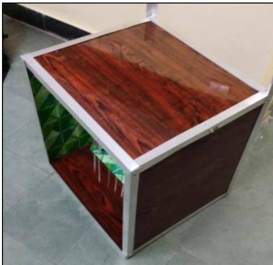
Figure 3 PCM based air cooler in different orientations.
