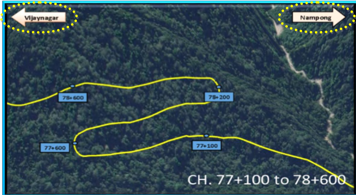
Figure 12 (b): “Hair Pin Zone Portions” in BRO – Nampong to Vijaynagar Roads, for Arunachal Pradesh (CH. 77+100 to 78+600).
