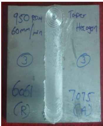
Figure.6. Tool: Hexagon. Side: Al6061 on retreating side and Al7075 on advanced side
