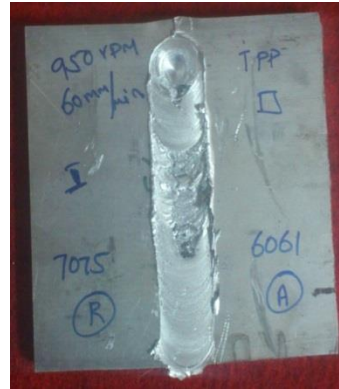
Figure.3. Tool: Square. Side: Al7075 on retreating side and Al6061 on advanced side
