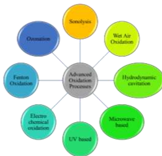
Figure 3: Representation of different AOPs applied for landfill leachate treatment
