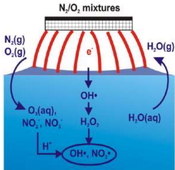
Figure 8: The schematic of plasma and its species generation. The image is reprinted from the literature [49].
