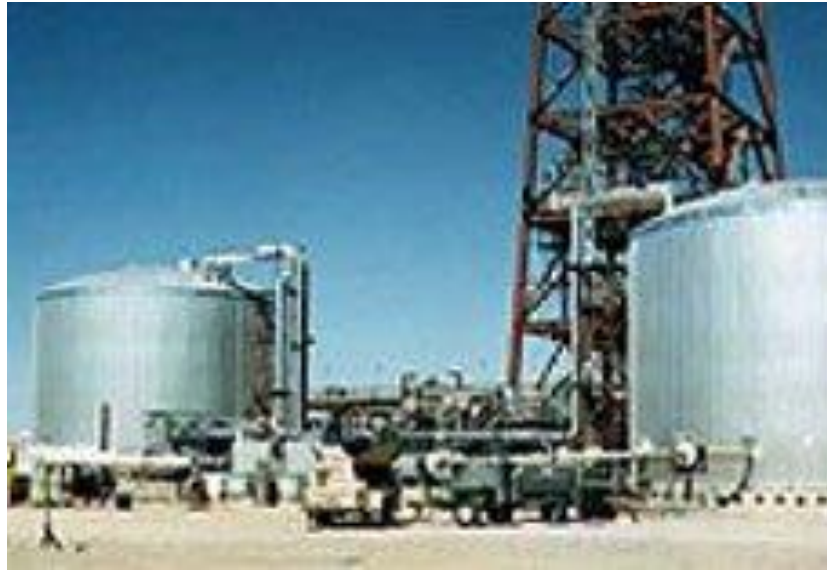
TWO-TANK DIRECT SYSTEM
