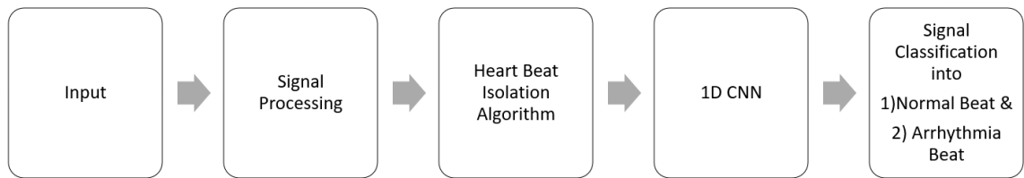
Fig. 4. Block diagram for the working of Arrhythmia Detection using Deep Learning Algorithms
