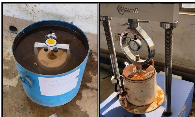
Figure 1: Soaked CBR Test setup.
