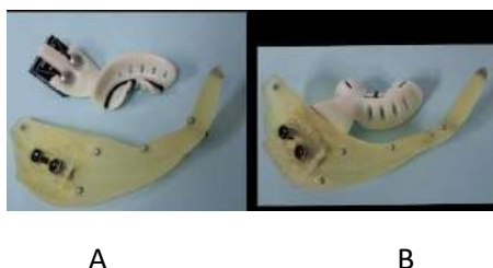
FIGURE (13A)- Yomi patient splint, shown with contrasting insert and fiducial array. (13B)- Yomi fiducial array, connected to patient splint.
