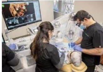
FIGURE16- Yomi Robotic operatory setup: Robotic guidance is delivered to the handpiece as haptic boundaries allows surgeon to maintain direct visualisation of surgical site. Note that the monitor provides visual confirmation as needed, while robotic haptics stabilize handpiece.
