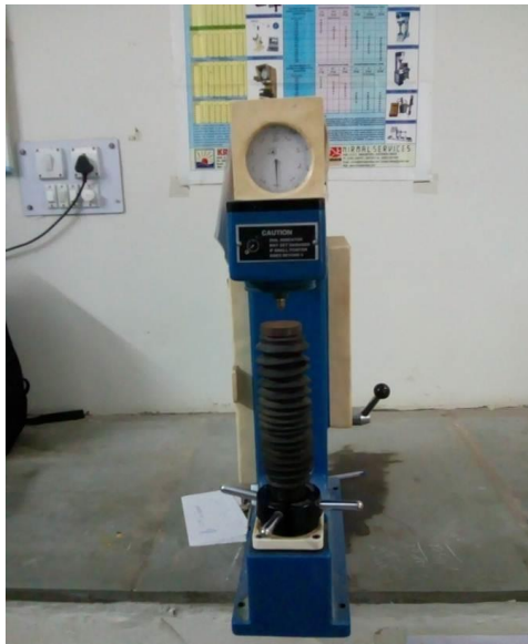
Figure 4 Hardness tester used for Brinell harness number measurement
