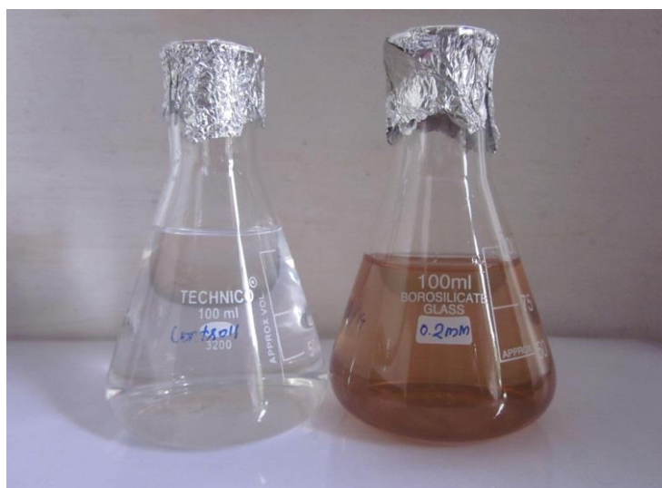
Fig .2: Conical flasks containing the aqueous extract before to (left flask) and following the 12-hour reaction with \text{Ag}^+ (right flask).
