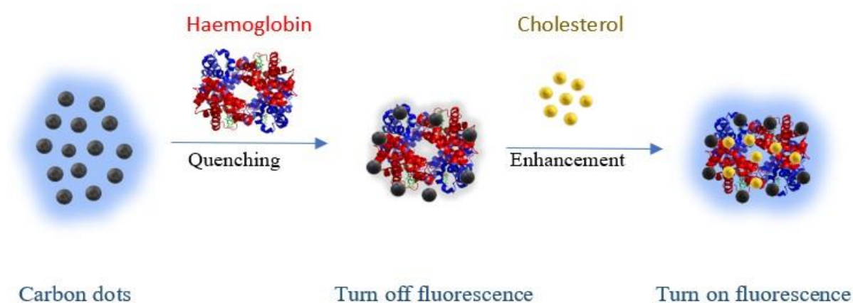
Fig 12. Pictorial representation of Cholesterol biosensor detection by the formation of CD-Haemoglobin complex
