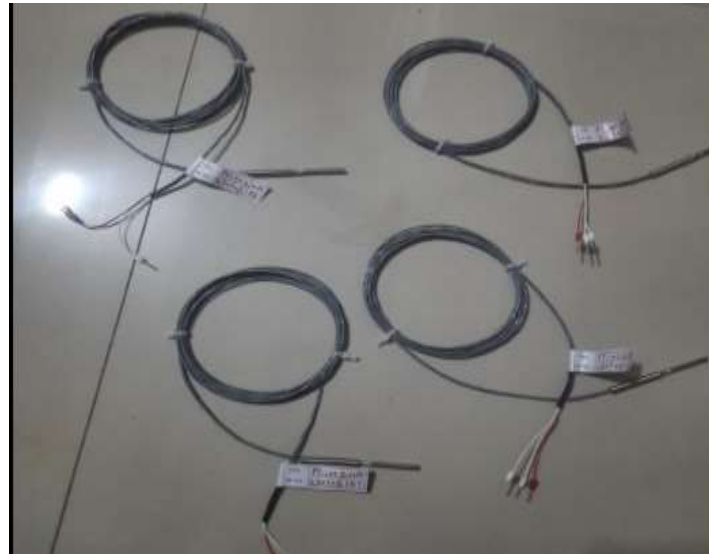
Figures 02 PT 100 Sensors used with multipoint temp indicator
