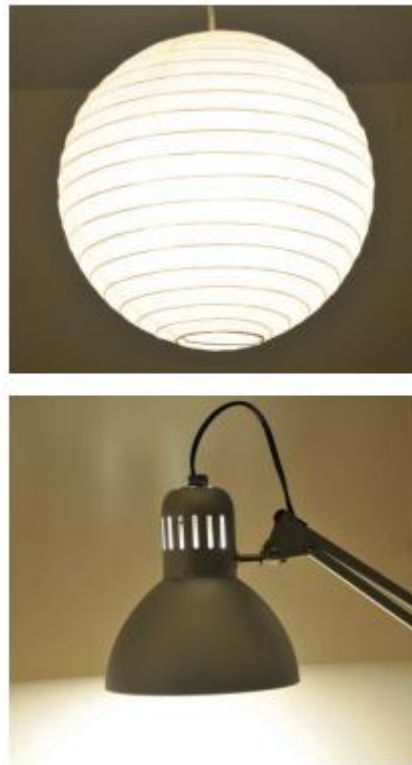
Figure 19. A diffusing shade produces an almost equal quantity of light in all directions (top). This kind of luminaire is often referred to as dispersive, because there is no directional quality to the light. The same light source can be surrounded by a metal shade or reflector to create a directional luminaire (bottom). The distinction between nondirectional and directional light is not the light source, but how it is used in the luminaire. [Source: Lighting for Interior Design]
