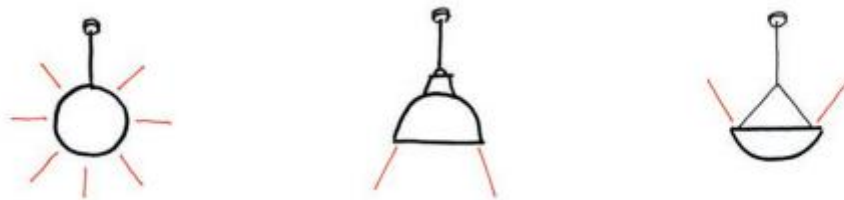
Figure 29. Left: Non- Directional Pendant; Center: Downlight Pendant; Right: Uplight Pendant[Source: Lighting for Interior Design]
