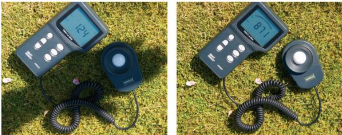
Figure 8. Even in the shade, on a sunny day there is a lot of ambient light around—12,400 lux (1,152 fc) in the measurement shown on the left. Nevertheless, this figure is less than one-seventh of the 87,100 lux (8,092 fc) measured from the direct sunlight on the right. A 7:1 variation in light levels over such a small distance would normally be designed out of the lighting of an interior space, yet this extreme contrast is exactly what natural light is all about. [Source: Lighting for Interior Design Book]
