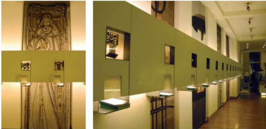
Figure 20. Concealed lighting is mounted within a linear display band. [Source: Lighting for Interior Design]
