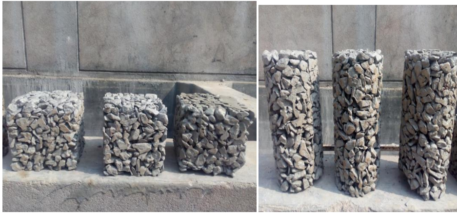
Figure 1. Cubes and cylinder specimens of pervious concrete
