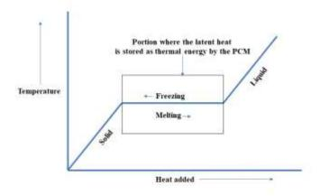
Fig. 1 Functioning of PCM as LHS.
