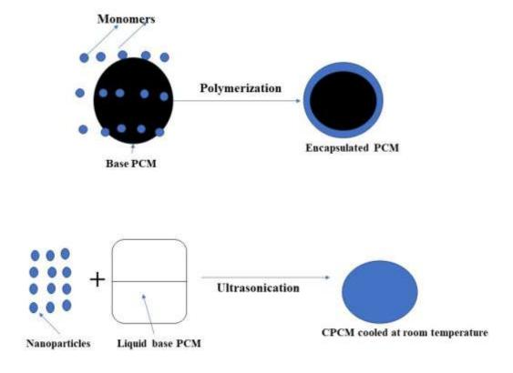
Fig. 2 Basic schemes of adding nanoparticles to the base PCM.
