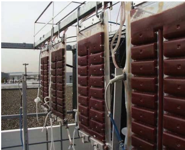
Fig. 4 Flat panel airlift from Subitec [38, 102] with usage of the flashing light effect, here for astaxanthin production
