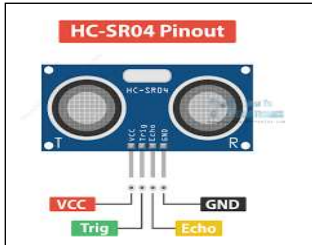
Figure 8: Ultrasonic Sensors HC – SR04
