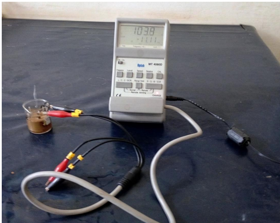
Fig.2 Static dielectric constant measurement setup
