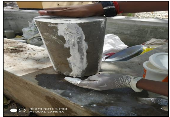
Figure2. Cylinder repairing process
