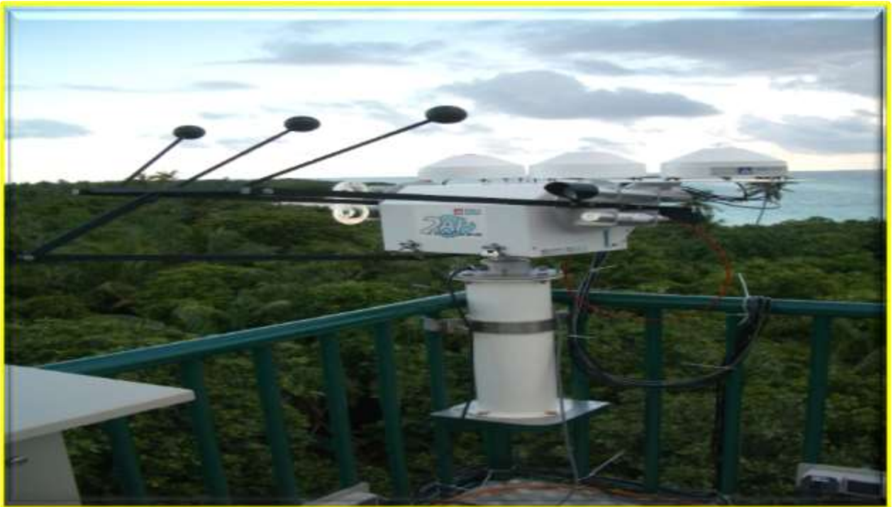
Sun Shine OR Intense Insolation Recorder Installed for Measurement @ Observatory Tower – 2.
