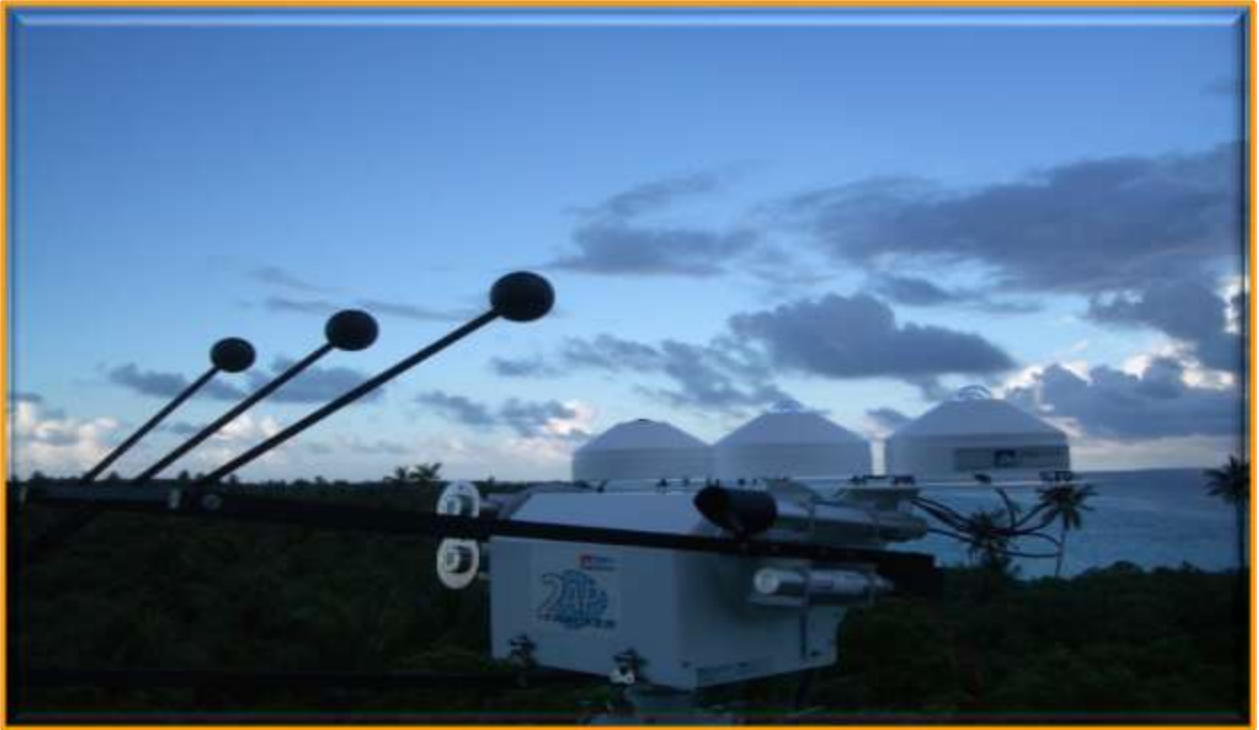
Sun Shine OR Intense Insolation Recorder Installed for Measurement @ Observatory Tower – 1.
