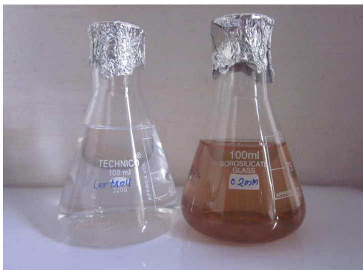
Fig .2. Conical flasks with the aqueous extract before (left flask) and after reaction with Ag + for 12 hrs(right flask).
