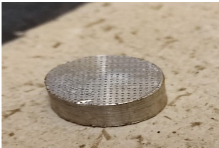
Fig. 4 Surface Texturing pattern on specimen
