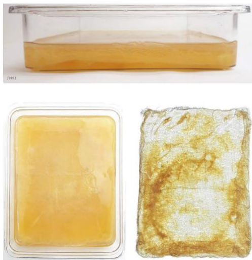
Fig. 30 : Bacterial cellulose on cotton gauze (source : Design Potential of Microbial Cellulose in Growing Architecture, Maters' thesis, Karolina Bloch 2019)
