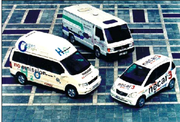
Gaseous hydrogen fueled Nekar 1 (1994) and Nekar 2 (1996), and liquid methanol fueled Nekar 3 (1997).
