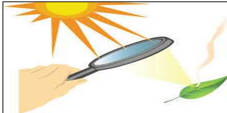
Figure 1: The magnifying glass converge the sunrays to a focal point on a leaf converting the energy of light waves to become hot enough to burn a leaf.
