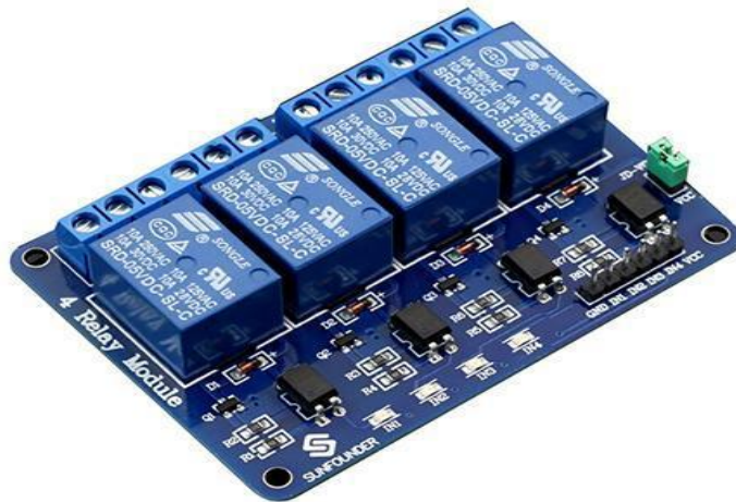
Figure 5.3: Relay with the driver circuit
