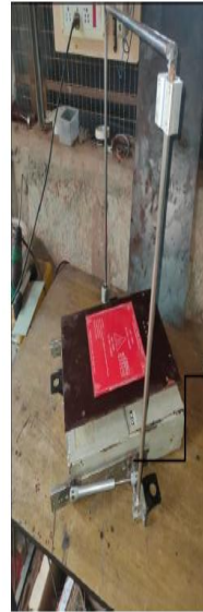
Z axis frame made of SS 12mm rod
