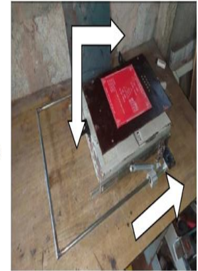
Z-axis frame mounted to base cabinet
