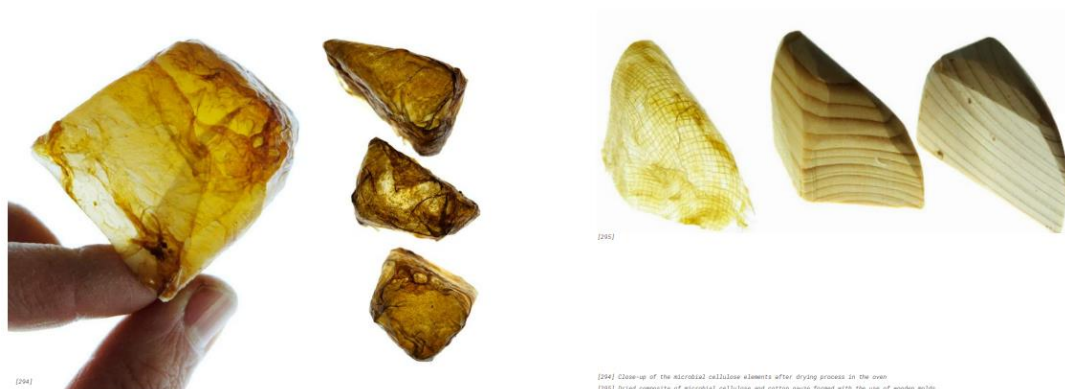
Fig. 32 : Bacterial cellulose on wooden piece and cotton fabric (source : Design Potential of Microbial Cellulose in Growing Architecture, Maters' thesis, Karolina Bloch 2019)
