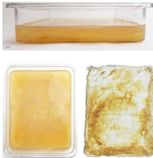
Fig. 30 : Bacterial cellulose on cotton gauze (source : Design Potential of Microbial Cellulose in Growing Architecture, Masters' thesis, Karolina Bloch 2019)
