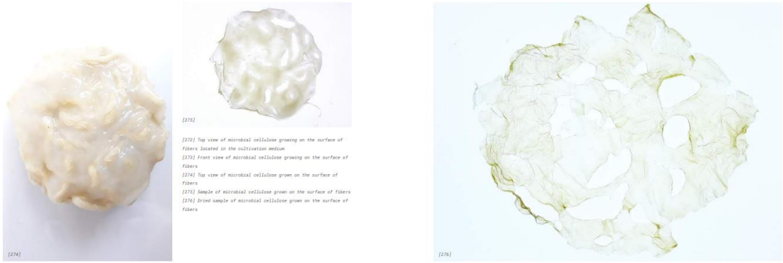
Fig. 21 : Top view of microbial cellulose growing on the surface of fibres located in the cultivation medium
