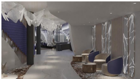
Figure 64 Winter season: The pattern on the louvers changes by using Electroluminescent ink (EL Print) which was applied to the textile by using a special inkjet printer
