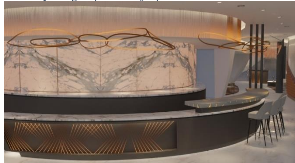
Figure 73 Lumi splash is a type of material that can change color and pattern and can illuminate. it is used with the marble pattern on the walls of the back counter of the bar and on some of the tabletops
