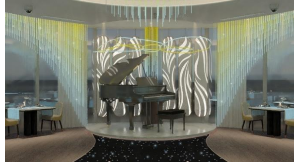
Figure 82 Floral pattern representing Spring is shown on the louvers behind the piano by using Electroluminescent ink
