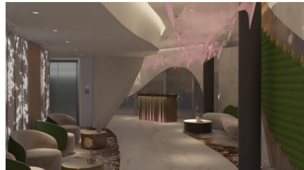
Figure 67 on the back of the chair, the upholstery used is smart fabric that can change color through heating thin metal wires that are incorporated within the fabric
