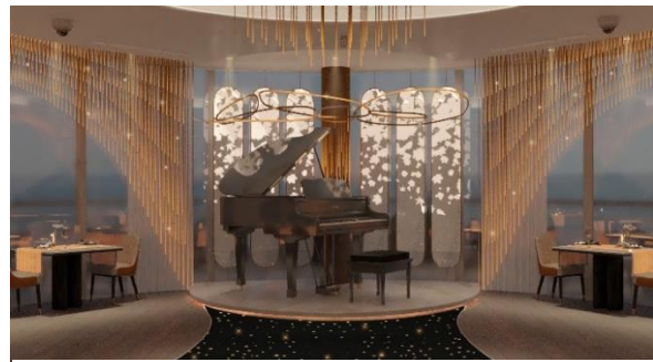
Figure 71 Falling leaves pattern representing Autumn is shown on the louvers behind the piano by using Electroluminescent ink (EL Print) which was applied to the textile by using a special inkjet printer
