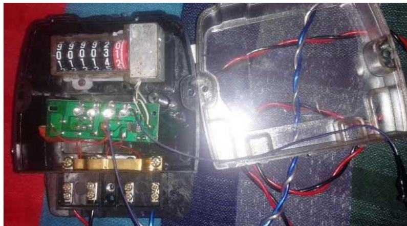
Figure.3 Connect Energy Meter with Arduino
